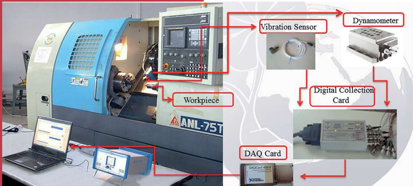
Figure 1: CNC turning machine that can make measurements with a vibration sensor and a dynamometer
