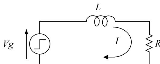
Figure 6 Lumped-parameter model of configuration of Figure 1
