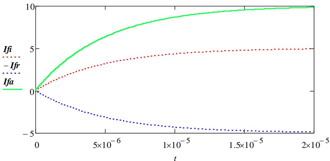
Figure 4 Response of a short-circuited line over a period of 20 micro-seconds
