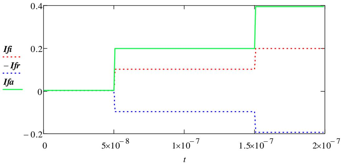
Figure 3 Response of a short-circuited line over a period of four traverses of the step
