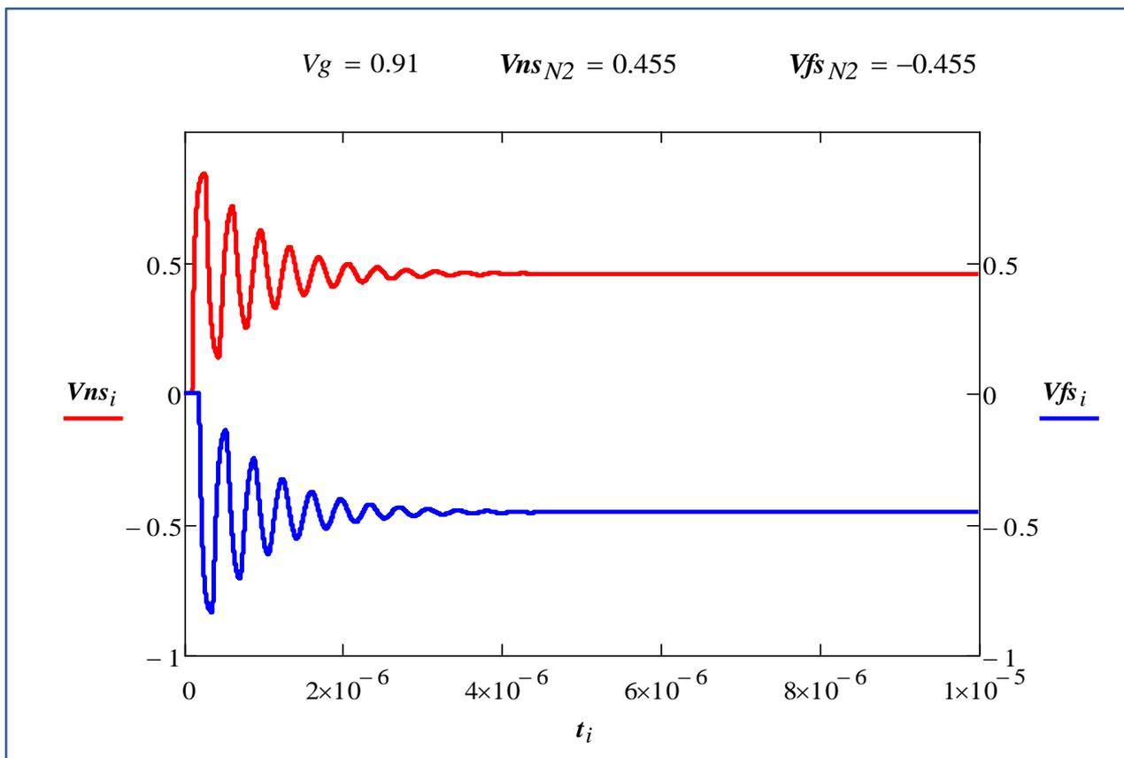
Figure 11 Waveforms of the voltages on the send and return conductors.
