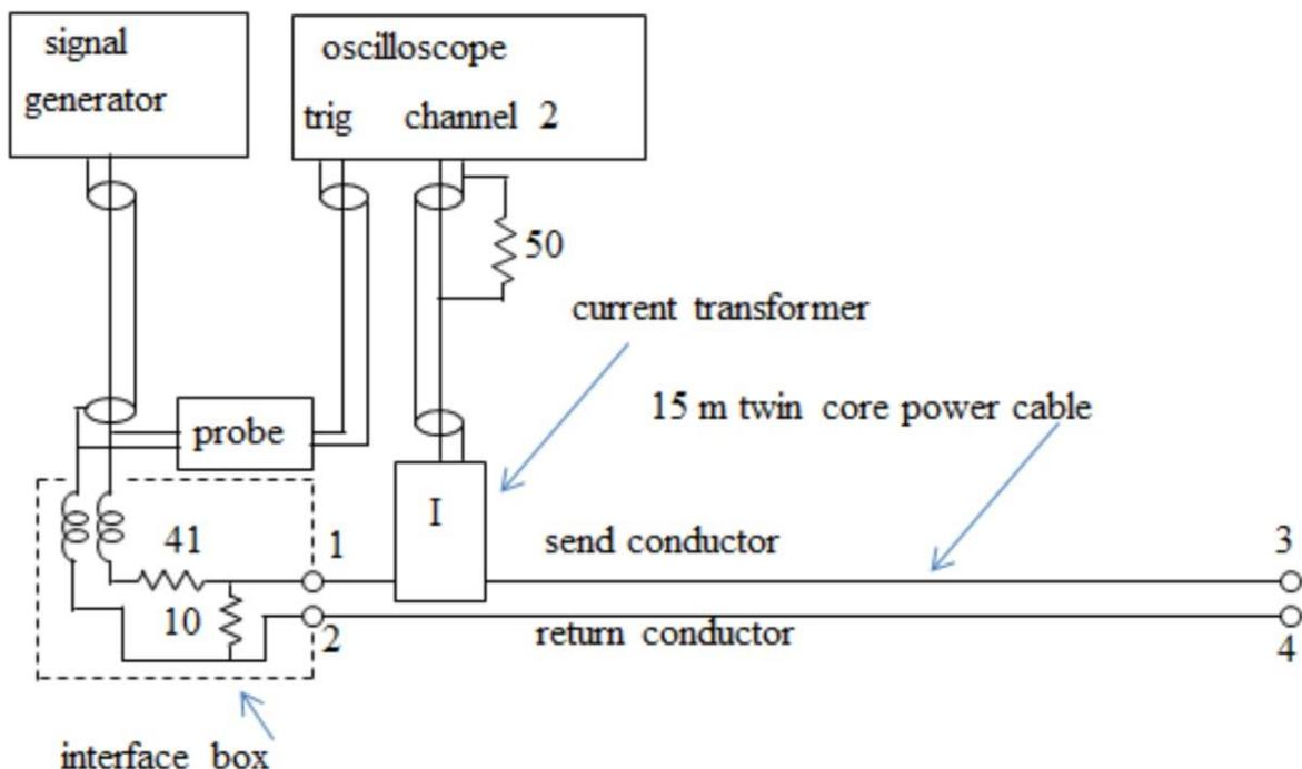
Figure 1 Setup used to investigate the transient response of twin-conductor cable.
