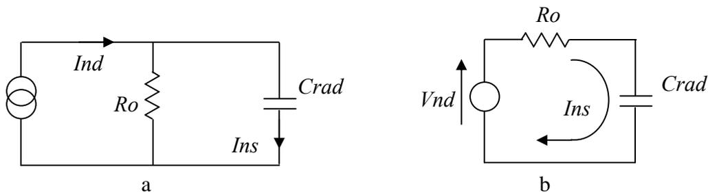
Figure 6 Deriving the amplitude of the discharge current  $I_{ns}$
