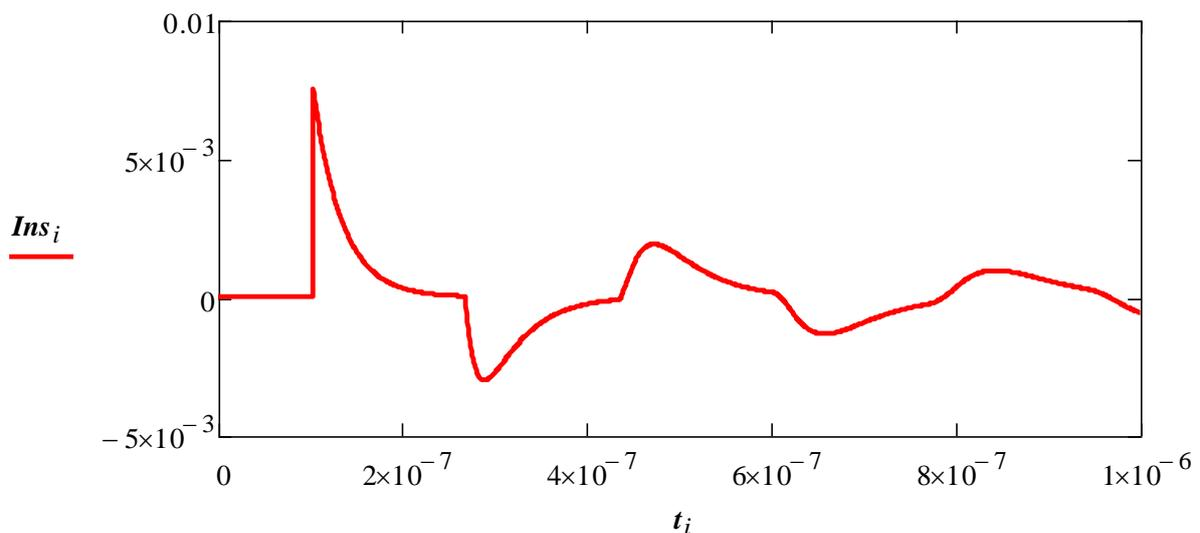
Figure 10 Waveform of the transient emission from the cable
