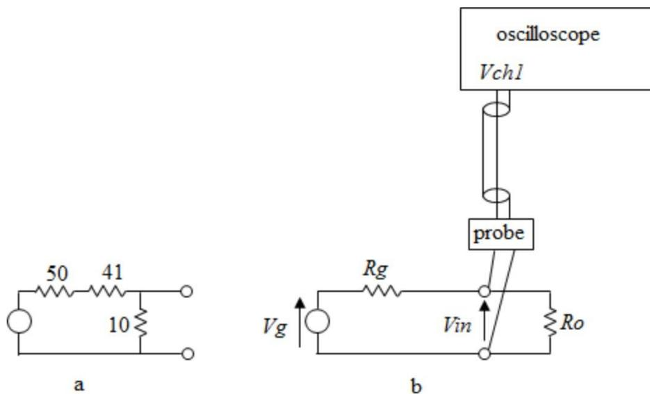
Figure 3 Circuit model of input circuitry
