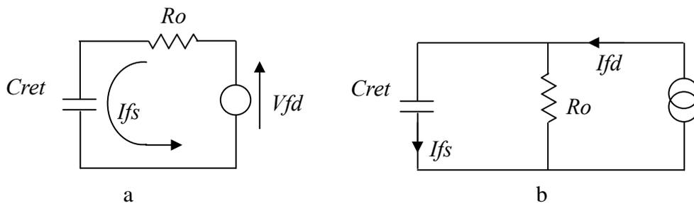
Figure 7 Deriving the amplitude of the recharge current  $I_{fs}$
