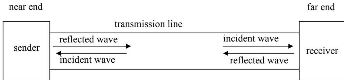
Figure 3 Block diagram illustrating the propagation of electromagnetic energy.
