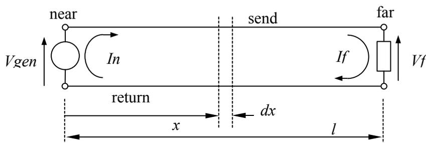
Figure 1 Schematic diagram of a twin conductor transmission line
