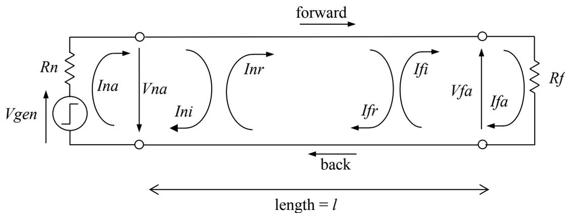
Figure 4 Delay line model
