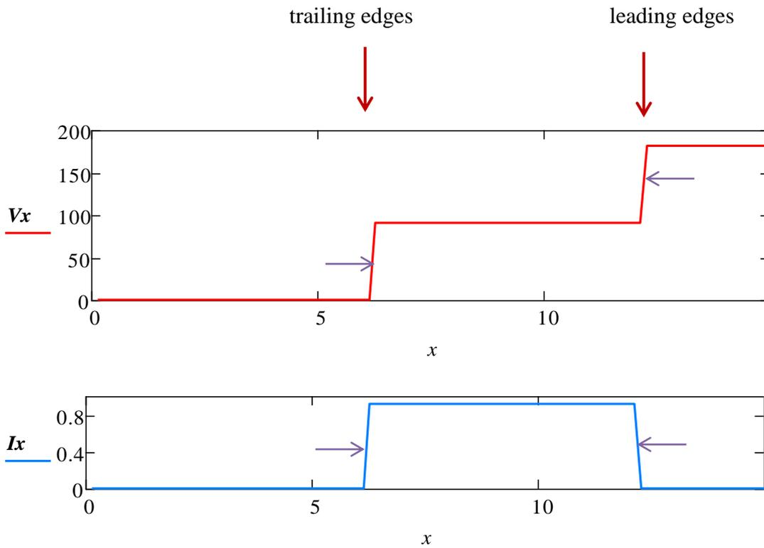
Figure 7 Distribution of voltage and current at  $t = 60\text{ns}$ . Far end open-circuit.
