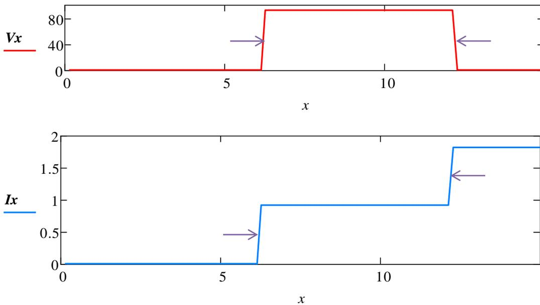
Figure 7 Distribution of voltage and current at  $t = 60\text{ns}$ . Far end short-circuit
