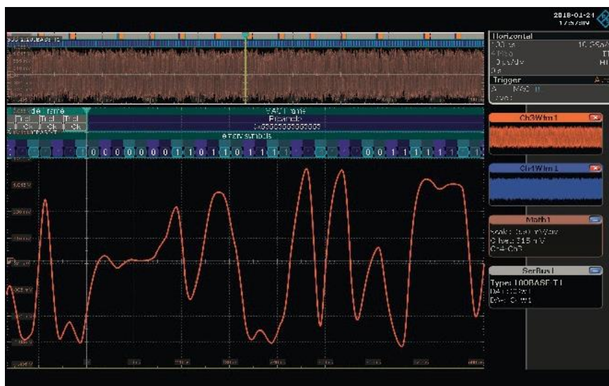
Figure 1: (top) A differential 100BASE-Tx signal, showing its three levels and the steep edges at the signal transitions; (bottom): An automotive 100BASE-T1 signal, showing how pre-distortion masks the three levels of the PAM-3 signal
