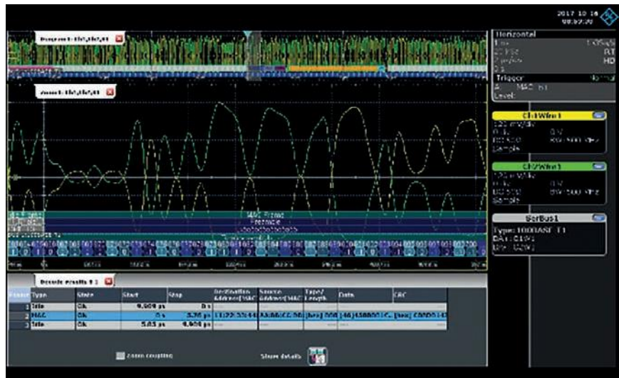
Figure 4: This screenshot shows the two levels of the differential 100BASE-T1 signal correlated with the decoded telegram content
