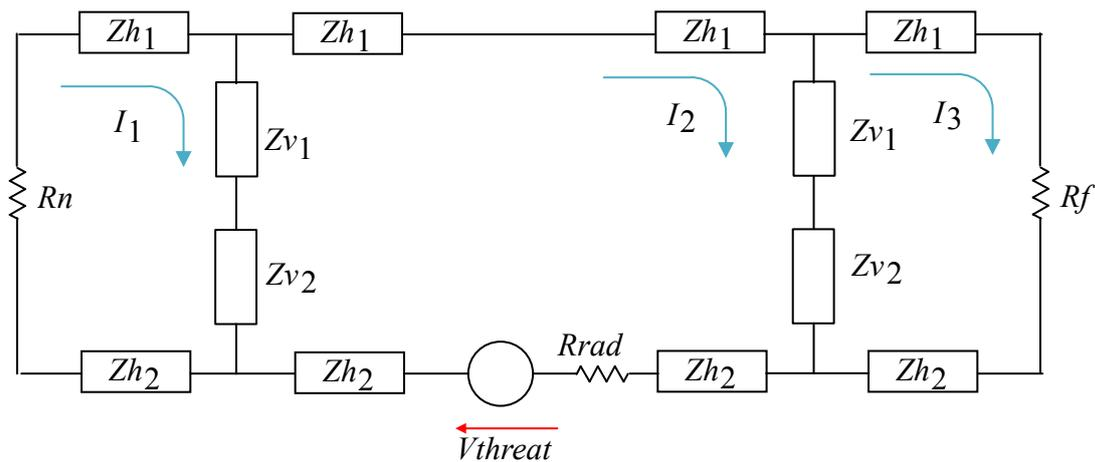
Figure 9 Simulating the response of a twin conductor line to external interference
