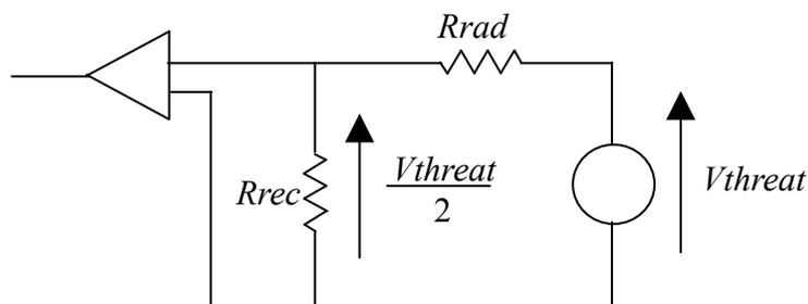
Figure 6 Circuit model of receiver assembly
