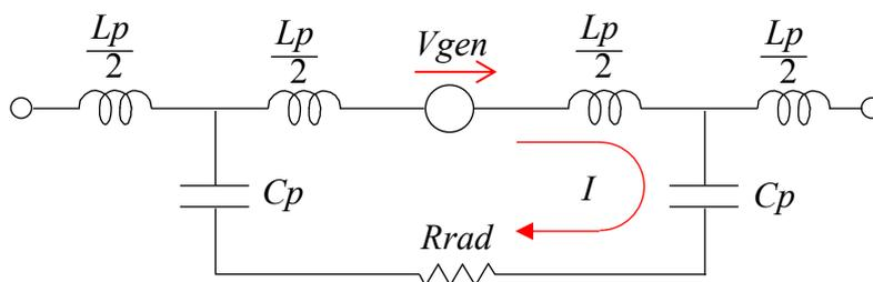
Figure 1 Simulating radiated emission
