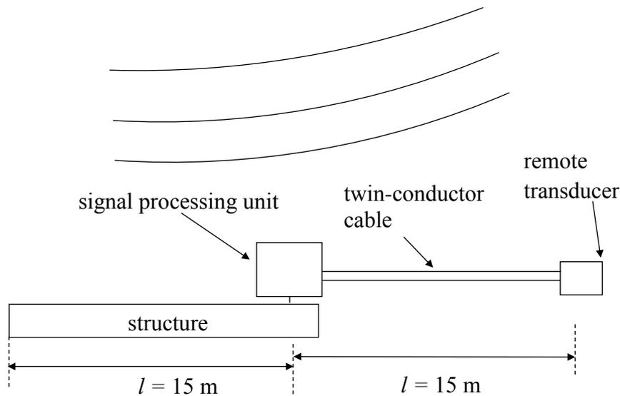
Figure 7 Cable exposed to external radiation
