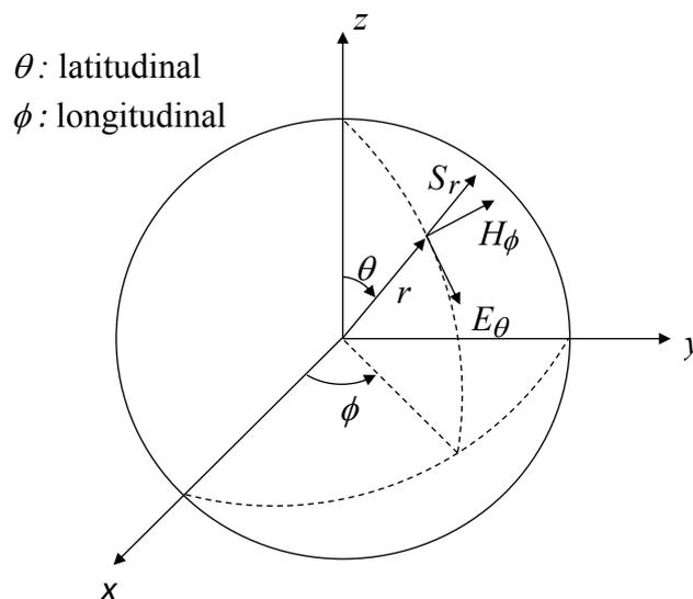
Figure 2 Power density on a spherical surface.
