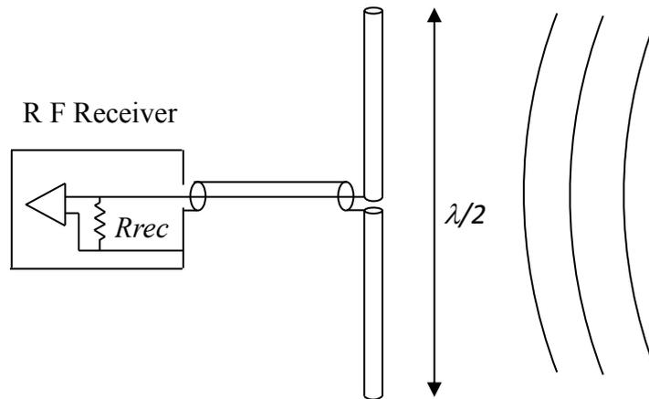
Figure 5 Illustration of a receiver assembly
