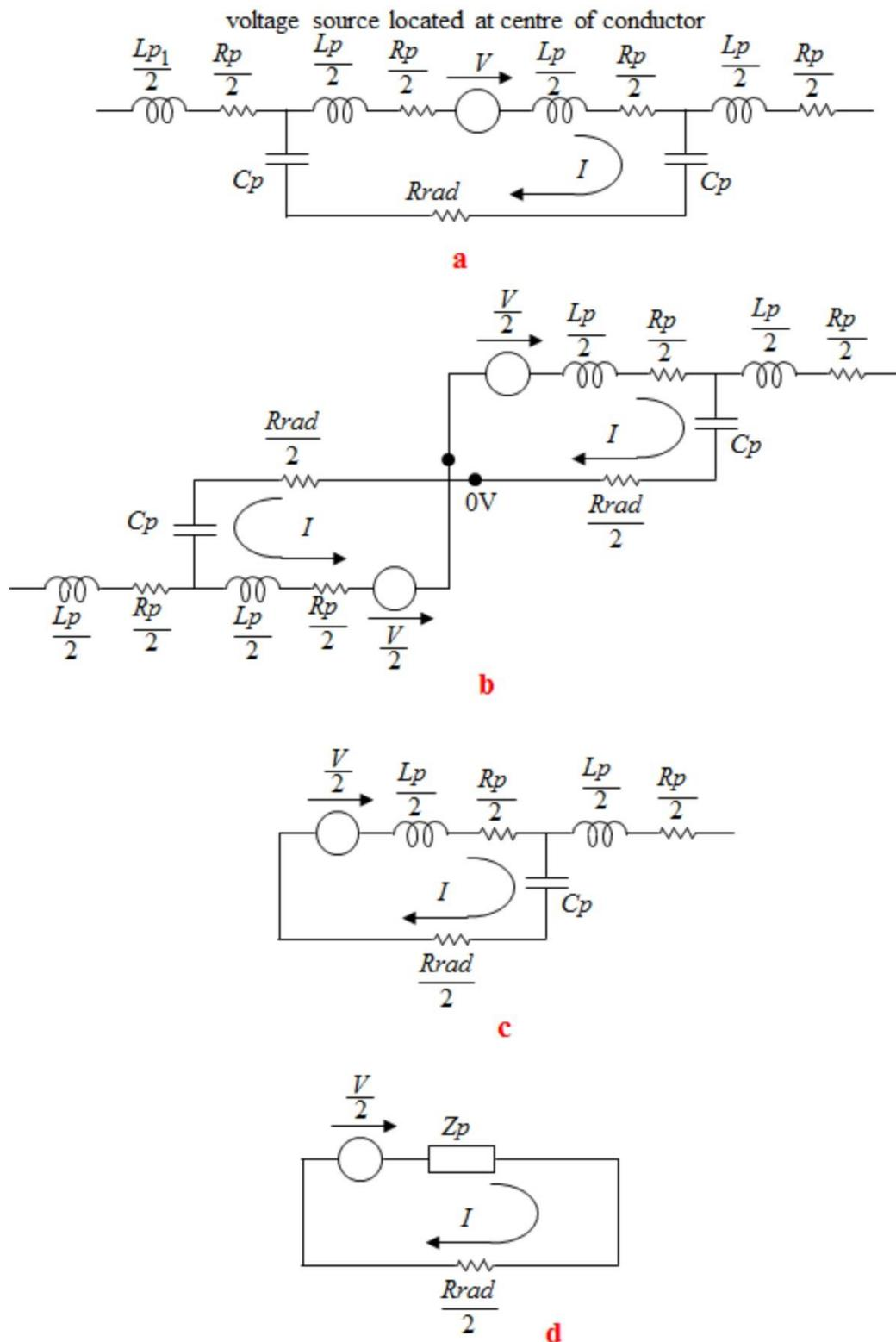
Figure 1 Simplifying the model of a single conductor
