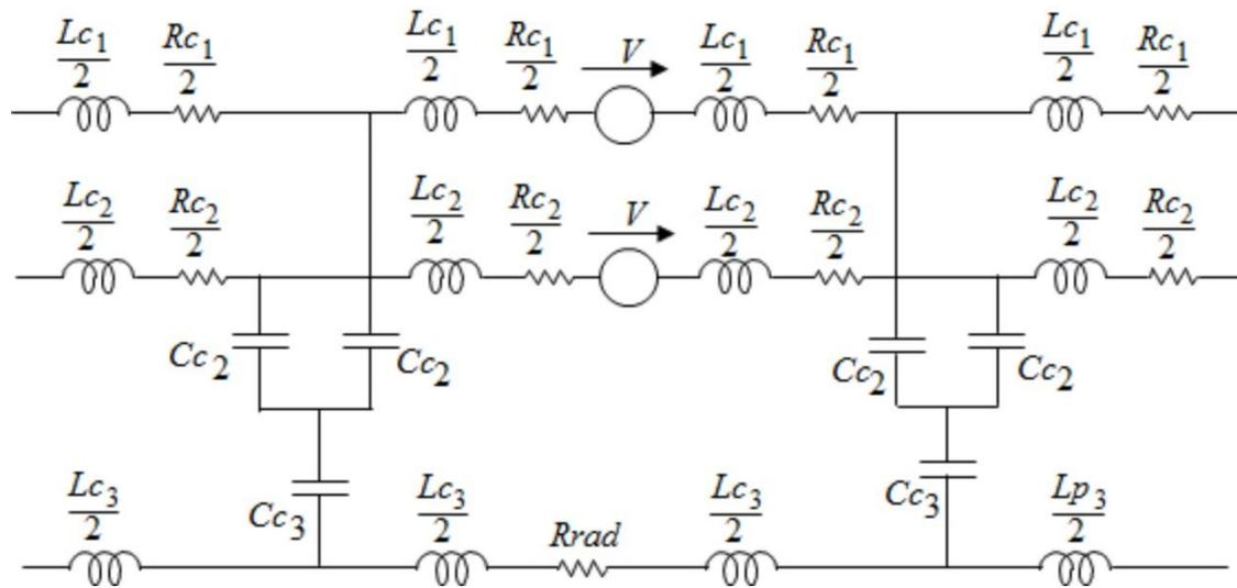
Figure 3 Complete circuit model of a twin conductor assembly
