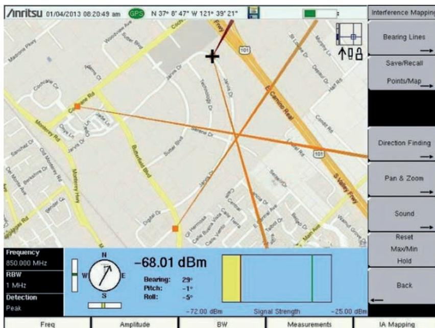
Figure 6: Interference mapping option of the MS2720T spectrum analyser showing three different azimuths intersecting at the suspected position of the interferer
