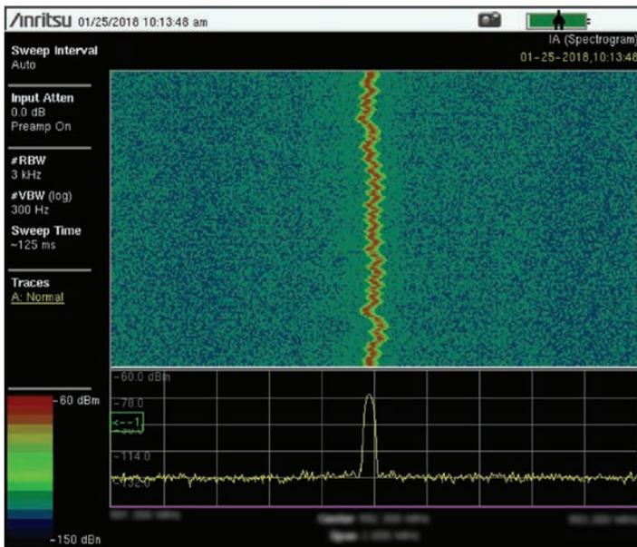
Figure 1: “Waterfall” display (spectrogram) showing frequency drift of a carrier
