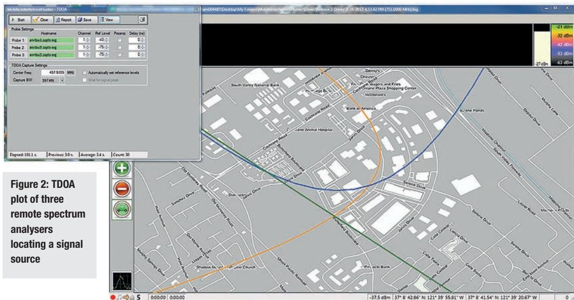
Figure 2: TDOA plot of three remote spectrum analysers locating a signal source
