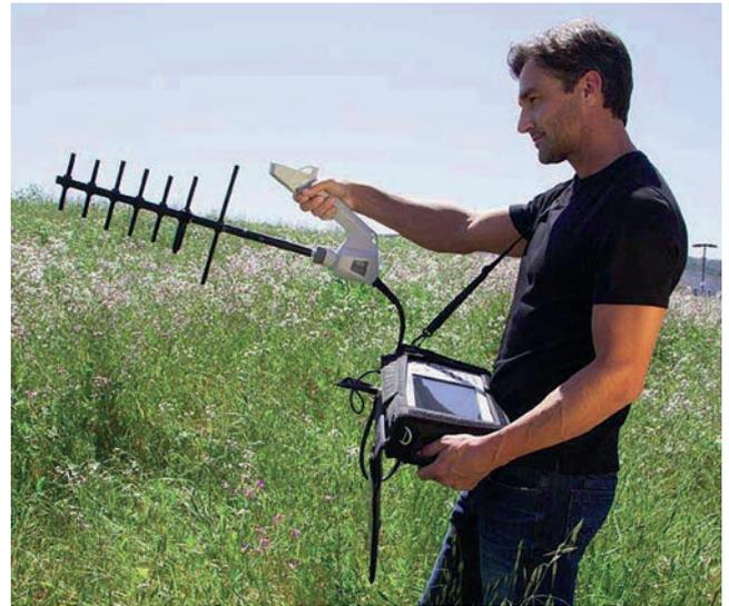
Figure 5: Directional antenna attached to the handle of the Interference Hunter allowing the source of a signal to be located
