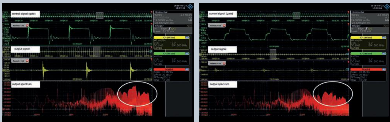
Figure 3: Comparison of standard square wave gate drive signal (left) with optimised gate drive signal (right). The lower red amplitude inside the white circle shows the significantly reduced emissions
