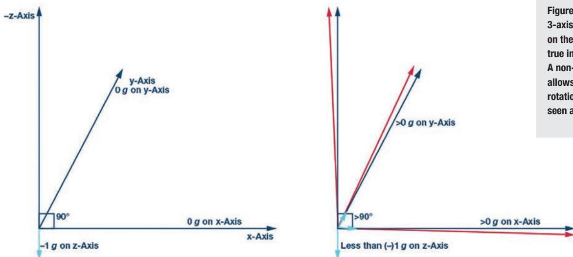
**Figure 1:** An ideal 3-axis orthogonal case on the left reflects the true impact of a vector. A non-orthogonal error allows leakage of rotation or force to be seen across all axes
