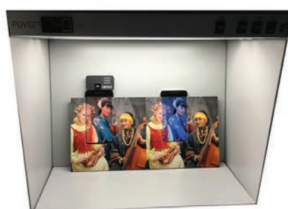
3,000K Color Temperature Fluorescent office light
