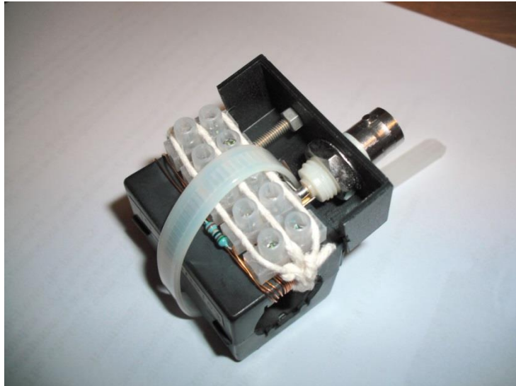
Figure 4 Current transformer assembly
