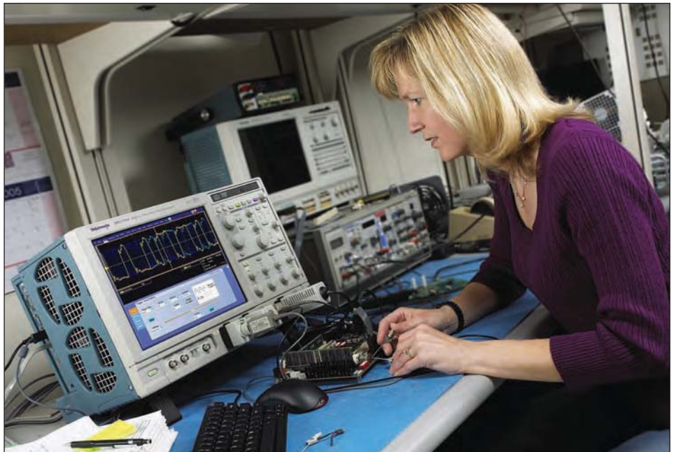
Figure 1: The Tektronix DPOPOWER power measurement and analysis software runs on the company's DPO7000 series of Digital Phosphor Oscilloscopes (DPOs)
