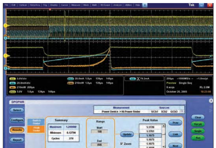
Figure 8: Using HiPower Finder and oscilloscope zoom for further analysis
