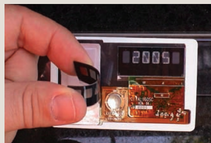
Figure 2: Citala's flexible display
