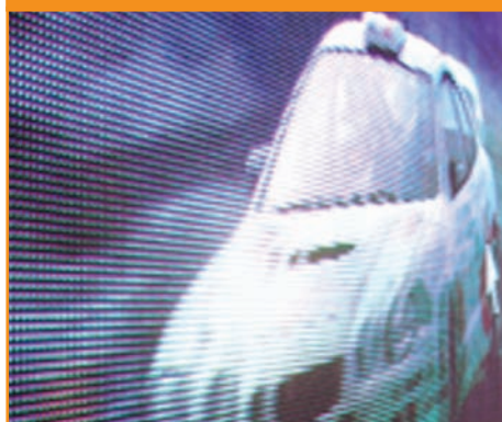
Figure 3 & 4: Multiple LEDs are mounted, with their packaged control electronics, as sub-assemblies on a tape assembly. Multiple tape assemblies are then joined together and a car image on one of these assemblies
