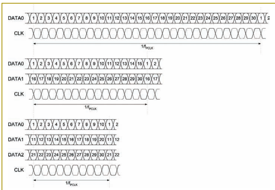
Figure 3: Serial transmission pixel clock referenced
