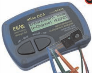
Atlas DCA Model DCA55 Semiconductor Analyser
