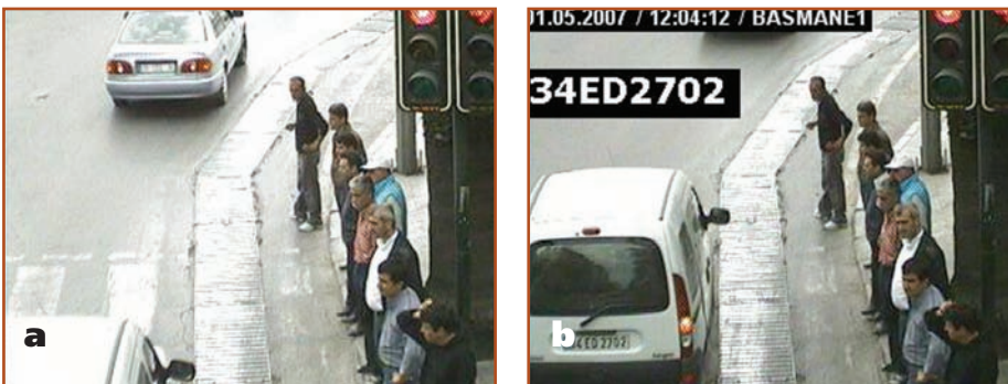
Figure 4: Pictures of a vehicle just before (a) and after (b) red light violation (red light violation system in Basmane-Izmir, Turkey)
