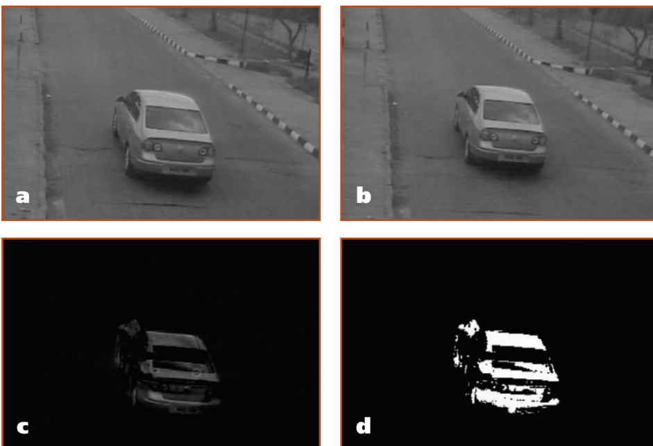
Figure 2: The current frame (a), previous frame (b), resulting difference image (c), binary image (d), obtained by thresholding the difference frame
