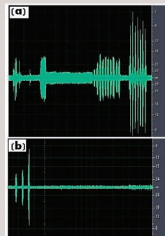
Comparison of sound recorded with a leading-edge commercial noise-suppression device to a recording with an ONFM
