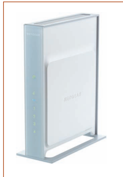
This wireless router from Netgear is powered by Marvell's TopDog 11n chip
