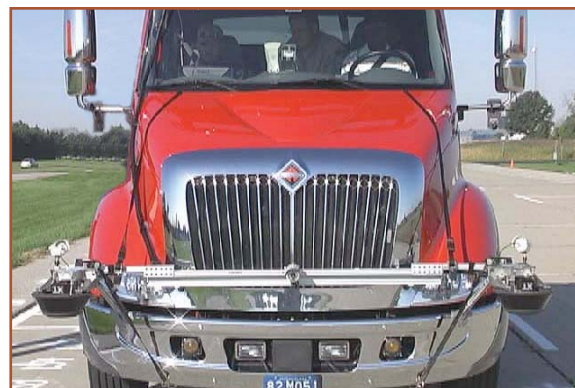
Truck cab instrumented for NIST tests of collision warning systems
