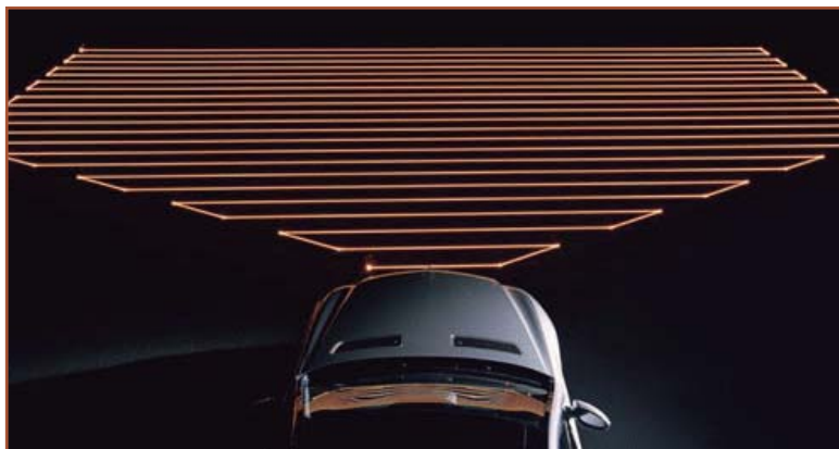
Short range radar observing the area in front of the motorcar.
