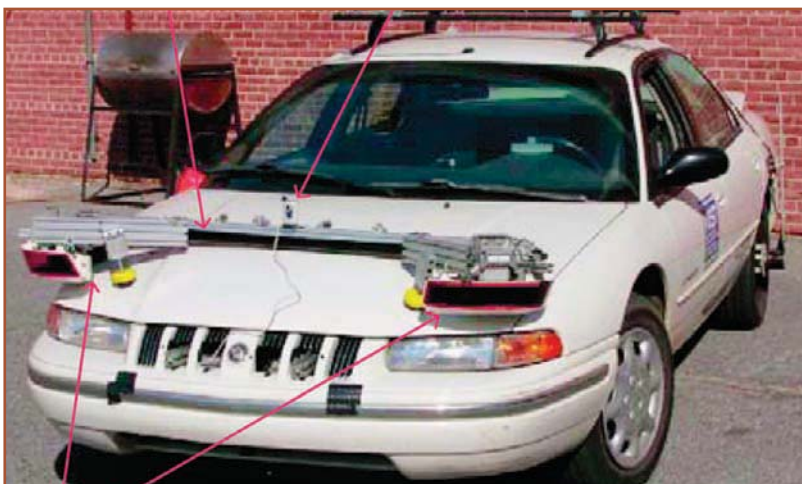
Test-bed vehicle with dual-head laser range scanner
