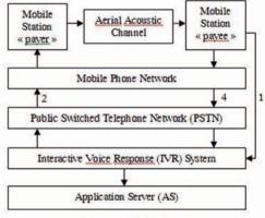
Figure 1: Face2Face<sup>TM</sup> overall architecture
