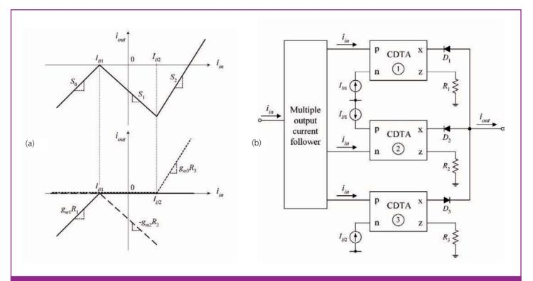
Figure 5: Piecewise-linear (PWL) function approximation function (a) desired transfer characteristic curve (b) circuit implementation
