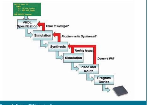
Figure 1: Outline FPGA design flow
