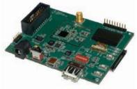
designs based on the Ripcord1 family of single-chip, all-CMOS Certified Wireless USB solutions.
