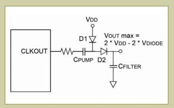
Figure 1: Typical charge pump
