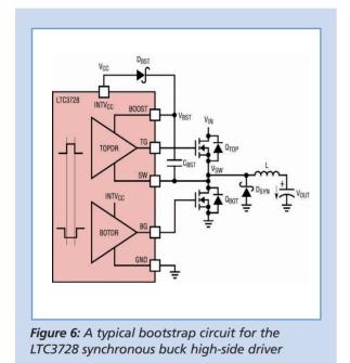
The bias voltage for the high-side driver is produced by the bootstrap supply circuit between the BOOST, INTVcc and SW pins. At the beginning of the initial cycle during startup, the SW pin is at zero voltage. The bootstrap capacitor is charged up to  $INTV_{CC}$  through diode  $D_{BST}$ .
