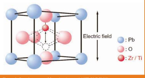
Figure 1: Crystal structure of ferroelectric material PZT (PB(ZrTi)O3)
