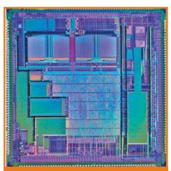
Figure 3: Silicon of the first FRAM embedded MCU from Fujitsu (MB95RV100)
