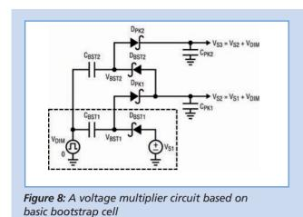
voltage on bootstrap capacitor  $V_{BST}$  is the sum of  $V_{DIM}$  and  $V_S$ , or in the LTC3728 buck application example,  $INTV_{CC} + V_{IN}.$  By adding one more diode and capacitor, a peak detector circuit can provide a voltage source equal to  $V_S + V_{DIM}.$
