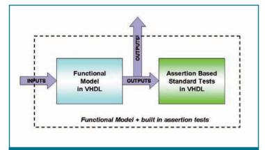
Figure 2: Extending model behaviour using assertions
