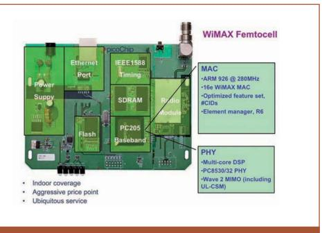
The company's femtocell architecture can be applied to both cellular and WiMAX air interfaces
