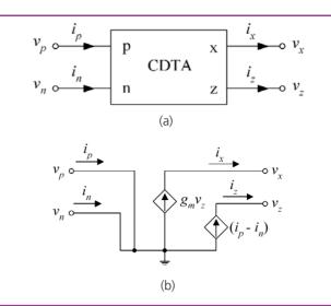
Figure 1: CDTA (a) circuit symbol (b) equivalent circuit
