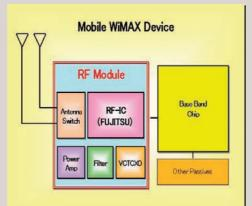
Block diagram of Fujitsu's WiMax IC solution
