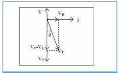
*Figure 2: Phasor diagram of capacitor equivalent circuit*
