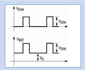
Figure 7b: Key waveforms of bootstrap circuit
