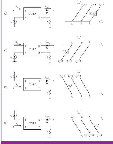
Figure 2: Proposed CDTA-based current limiter building blocks
