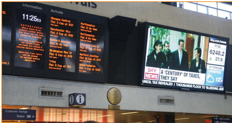
This picture, taken at Euston station, shows that a well-designed LED video wall can overcome the problem of reflections off the front surface. Sadly, the lower cost LED displays mounted adjacent to the video wall are mounted inside protective boxes and, again, ambient light reflecting off the surface of these displays reduces the legibility of the text
