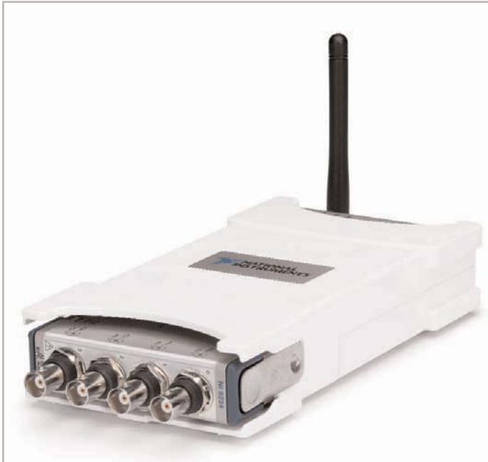
Figure 3: WLS-9163 containing NI-9234 dynamic signal acquisition module
