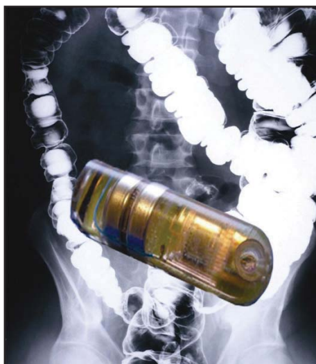
Lab-on-a-pill device for remote measurement of physiological conditions in the gut [Courtesy of the Royal Society of Chemistry]
