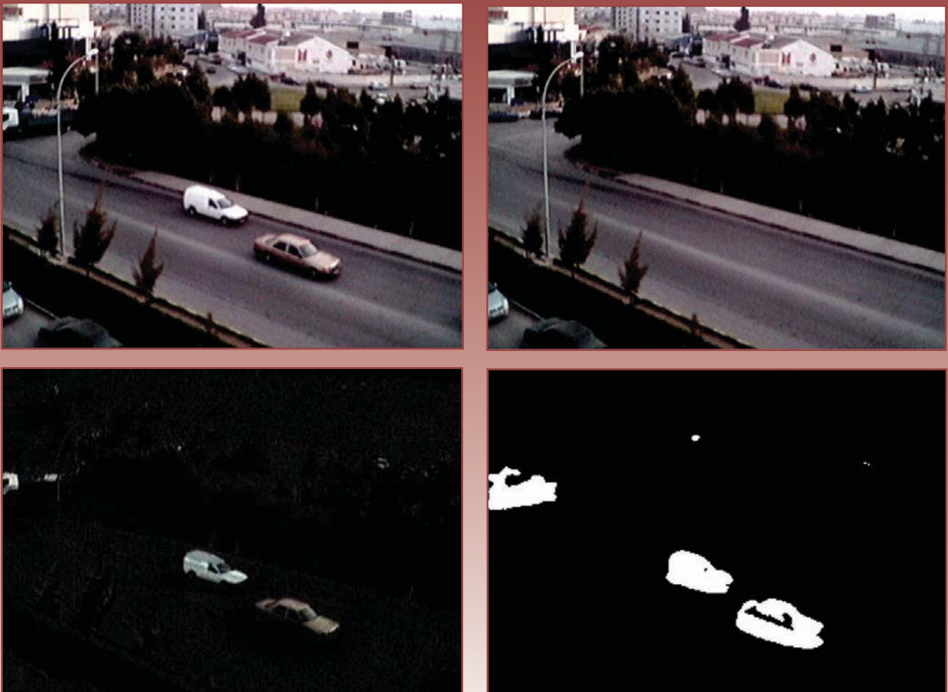
Figure 2: (a) current frame, (b) background image, (c) resulting difference image, (d) binary image obtained by thresholding the difference frame
