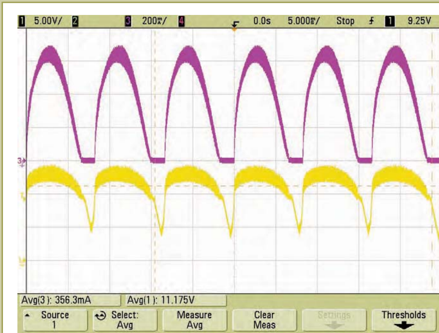
Figure 2: 120Hz AC LED current and voltage waveforms delivering ~ 4W of LED power
