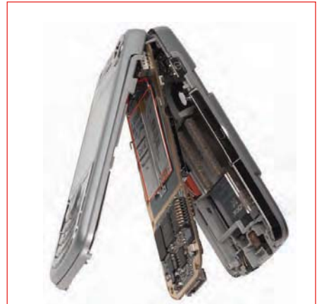
This phone has 1.2mm thick dual-cell supercapacitor to enable the BrightFlash feature; soon mobile phones will carry SMT supercapacitors too
