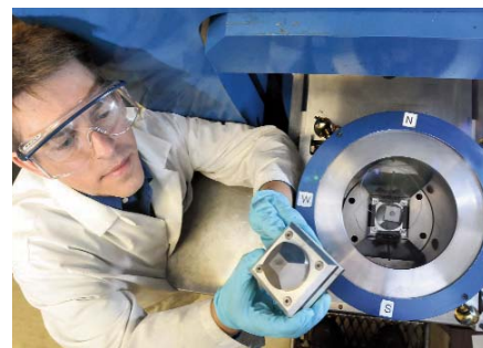
Argonne scientist John Mitchell assembles the high pressure furnace used in creating the multiferroic properties of \text{FeTiO}_3
