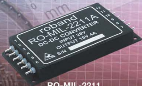
RO-MIL-2211 28V input 50W single output dc to dc converter 76.3x38.2x10.2mm, 60g
