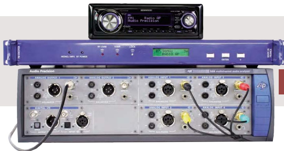
Figure 1: FM radio test setup, with APx526, transmitter and car stereo
