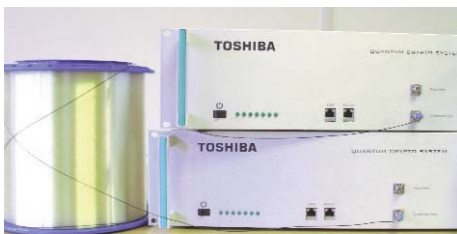
The Toshiba QKD system used to demonstrate 1Mb/s secure bit rate over 50km of fibre for the first time
