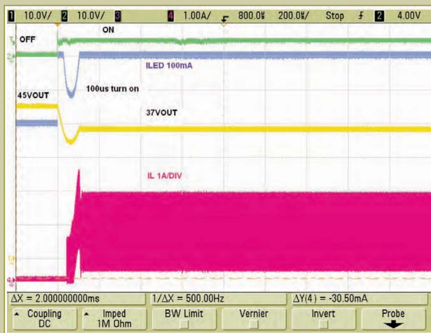
Figure 2a: Fast LED turn on using LED disconnect option 1 after 5s LED off
