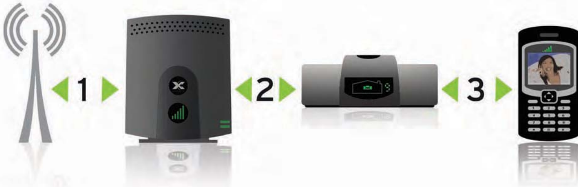
Figure 2: Bridging the gap between base station and handset
