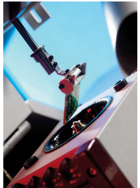
Solderability testing of electronic components
