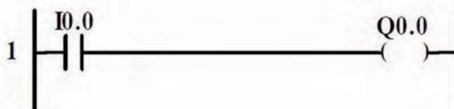
Figure 1: Ladder diagram for the user program UZAM_plc_8i8o_ex38.asm
