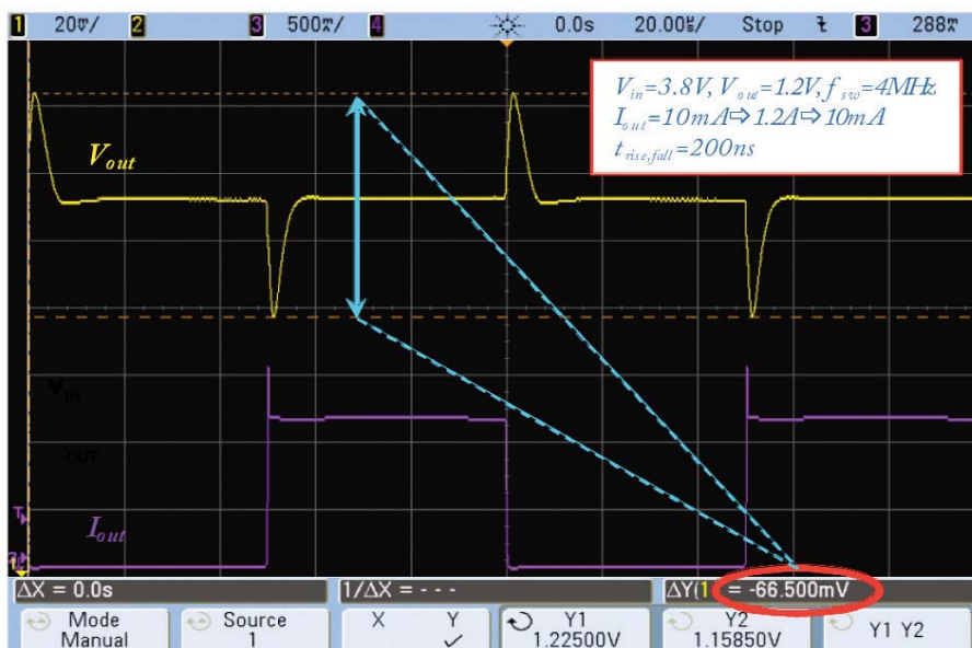
Figure 5: Transient performance of the Valley Mode Current Control WM8312 DC-DC
