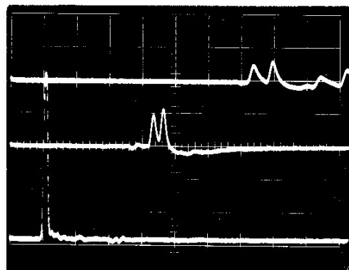
Figure 7: Signal on active left line with right line shorted to ground
