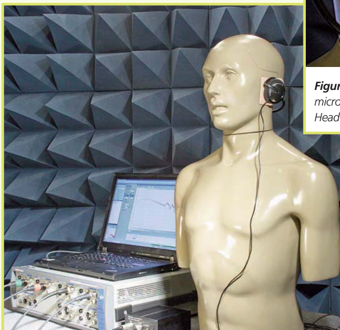
Figure 1: Testing headphones with a G.R.A.S. KEMAR 45BA mannequin and an Audio Precision APx526 analyzer
