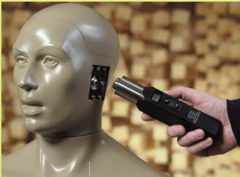
Figure 5: Calibrating the microphones
