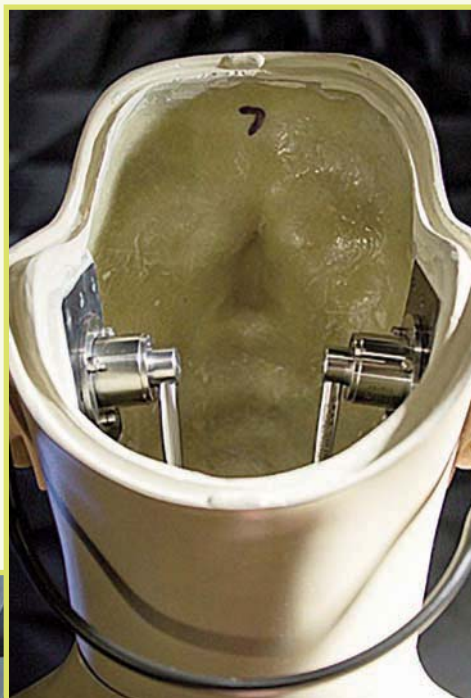
Figure 2: Ear simulators and microphones inside the head of the Head and Torso Simulator (HATS)
