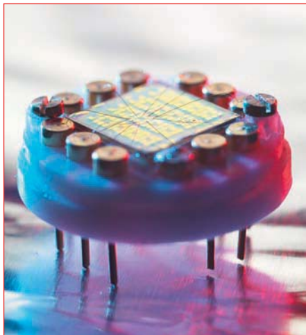
A light-sensitive graphene/polymer heterostructure
