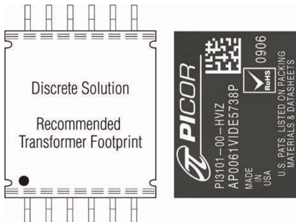
Figure 15: A module-based 60W total solution versus embedded solution recommended transformer size for a 40W solution
