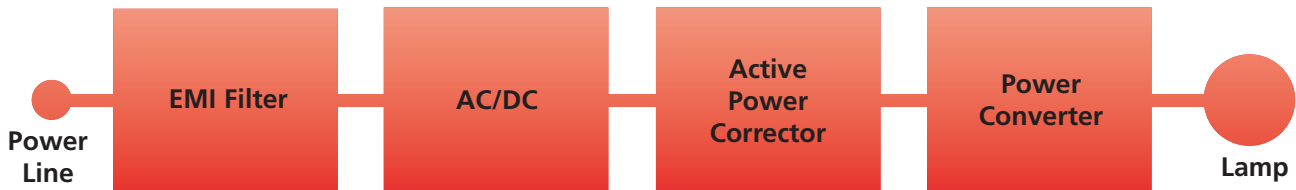
Figure 1: General lighting electronics block diagram
