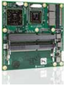
Figure 3: The Kontron microETXexpress-OH is a COM Express compact, Pin-out Type 6-compatible Computer-on-Module with CPUs from the new AMD G series range COM Express Computer-on-Modules
