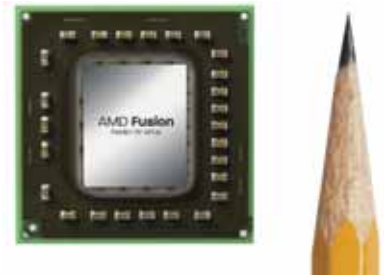
Figure 1: Within the compact footprint of only 19mm x 19mm, the new AMD embedded G-Series APU integrates a single-core or dual-core CPU, a programmable GPU, plus a video decoding unit and a memory and PCI Express controller on a single die
