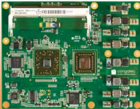
Figure 4: conga-BAF is the world's first COM Express basic Computer-On-Module which is based on the new AMD Embedded G-Series platform
