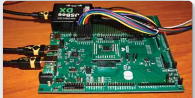
Figure 1: Connecting the USBee DX to the V2Eval board
