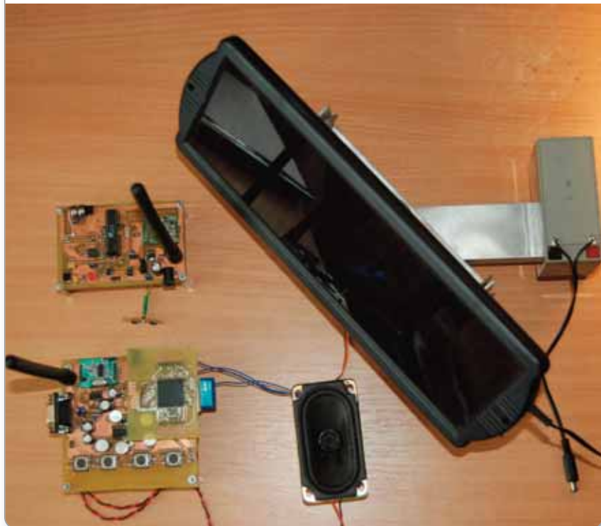
Figure 5: Photovoltaic power supply with sun-tracking for remote ambient temperature reading station
