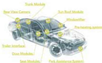
Selective ECU power switch-off helps save CO2 emissions and fuel consumption
