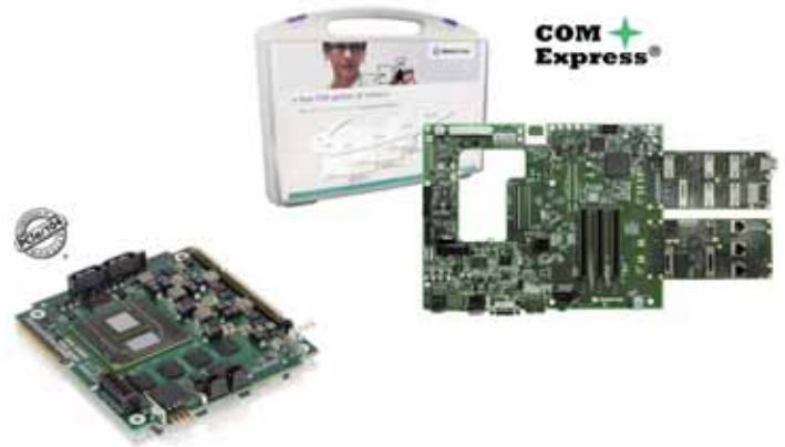
Figure 1: Current Kontron FPGA platforms: The PCIe/104™ Singleboard Computer Kontron MICROSPACE® MSMST with Intel® Atom™ E600C series processor and Altera Arria II GX FPGA on a multi-chip module and the Kontron COM Express™ FPGA Starterkit with Altera Cyclone IV GX FPGA
