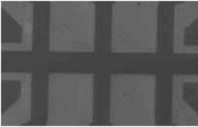
Scanning electron micrograph picture of graphene device. The dark area is monolayer graphene and the light areas is the silicon-carbide substrate
