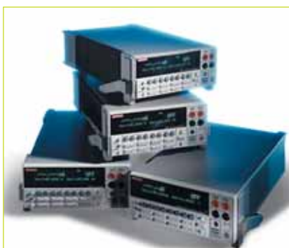
Figure 1: DC SMUs are a good choice for a variety of nano material and device test applications because they can switch rapidly between sourcing voltage/measuring current and sourcing current/measuring voltage
