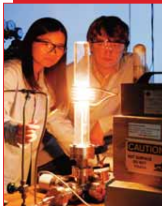
Georgia Tech graduate students Yike Hu and John Hankinson observe a furnace used to produce graphene on a silicon carbide wafer [Photo: Gary Meek]
