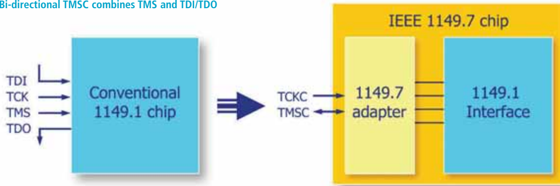
Figure 3: Bi-directional TMSC combines TMS and TDI/TDO
