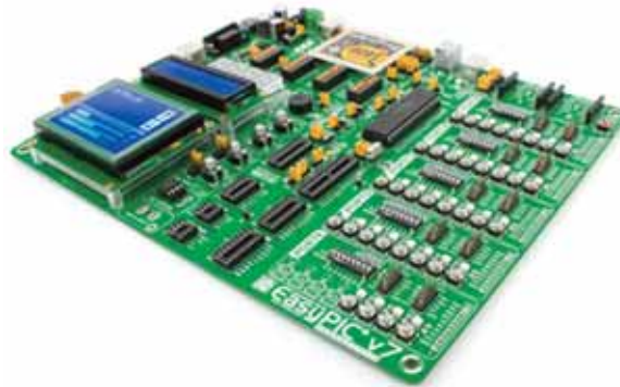
Figure 8: EasyPIC V7 microcontroller development board
