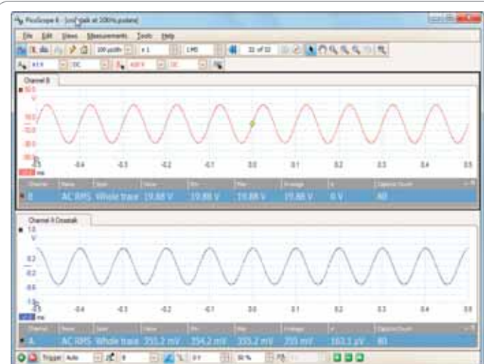
Figure 20: Upper view: left output channel driven at 10kHz; Lower view: right output, channel not driven
