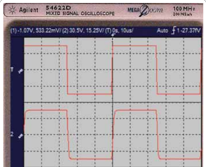
Figure 9(b): 20kHz square wave on 4Ω load
