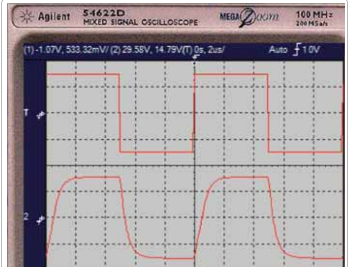
Figure 11(b): 100kHz square wave at 4Ω
