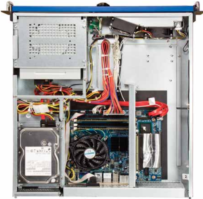
Figure 2: The component layout facilitates obstacle-free air circulation for efficient and quiet system cooling
