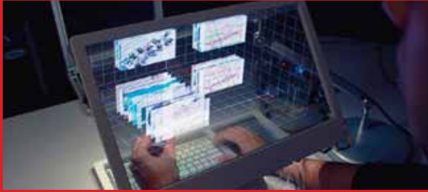
The SpaceTop 3D computer allows users to reach inside to manipulate files
