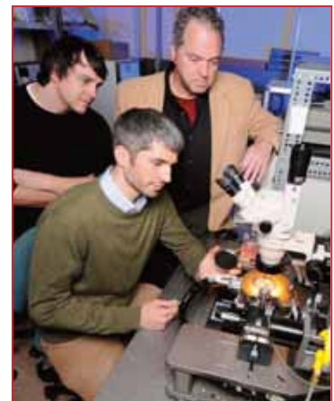
Georgia Tech Research Institute (GTRI) research engineers Kyle Davis and Ryan Westafer, with professor William Hunt of the School of Electrical and Computer Engineering (EC), examine a 3"-diameter silicon wafer on which they have fabricated thousands of bulk acoustic-wave devices capable of delaying electromagnetic waves (Credit: Gary Meek)
