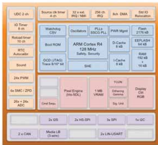
Figure 3: Block diagram of Fujitsu's single-chip solution for hybrid instrument clusters MB9EF226, also known as 'Titan'
