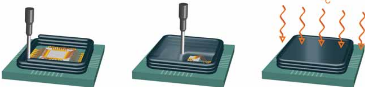
Figure 5: For "dam stacking", several adhesive beads are stacked and form a kind of wall. The volume within the wall can be completely filled with the low-viscosity encapsulant (fill). Afterwards, both compounds are cured in just one step
