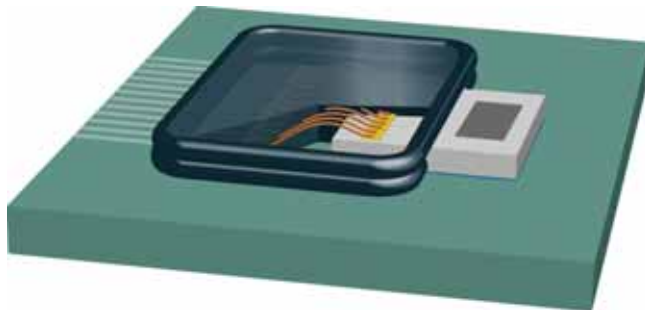
Figure 4: For partial encapsulation, only parts of the chips are covered by adhesive. In this case, it is particularly important that the adhesive cures at its intended position without flowing
