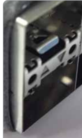
Figure 4: Close-up of the latch plate that includes the two thermal vent holes
