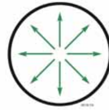
Figure 33: Forces that move the current density to the outside of a conductor are called skin effect
