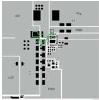
Figure 7: The hot loop of the LT3956 LED driver boost controller is shown in green
