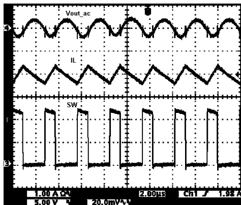
Figure 8: Working waveforms of the chip when V_{IN} = 12V , V_{OUT} = 3.3V , I_L = 2A
