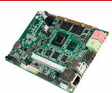
Figure 2: Qseven Computer-on-Module concept with carrier board and computer module
